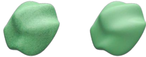
Figure 1. Comparison between a printed appearance (left)—highlighting its non-uniformities—and the computed ideal uniform (right).
