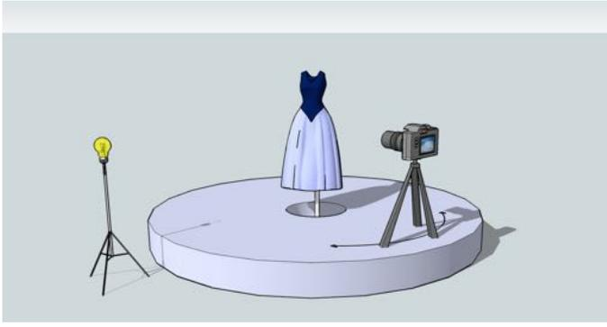
Fig. 4. The basic components of a capture environment. Ideally there should be several lights filling in all the shadowed areas on the object. The camera should be moved as opposed to the object.
